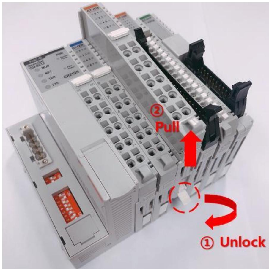
As above figure in order to safeguard the FnIO module from jamming, it should be fixed onto the DIN rail with locking level. To do so, fold on the upper of the locking lever.
